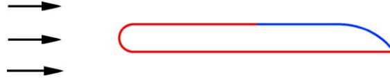
Figure 1. Blake airfoil used in unsteady laminar flow problem. The right half section of the upper surface is allowed to deform.
